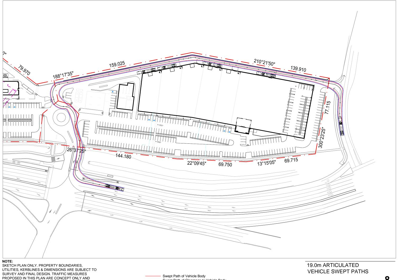
Swept Path of Vehicle Body Swept Path of Clearance to Vehicle Body
